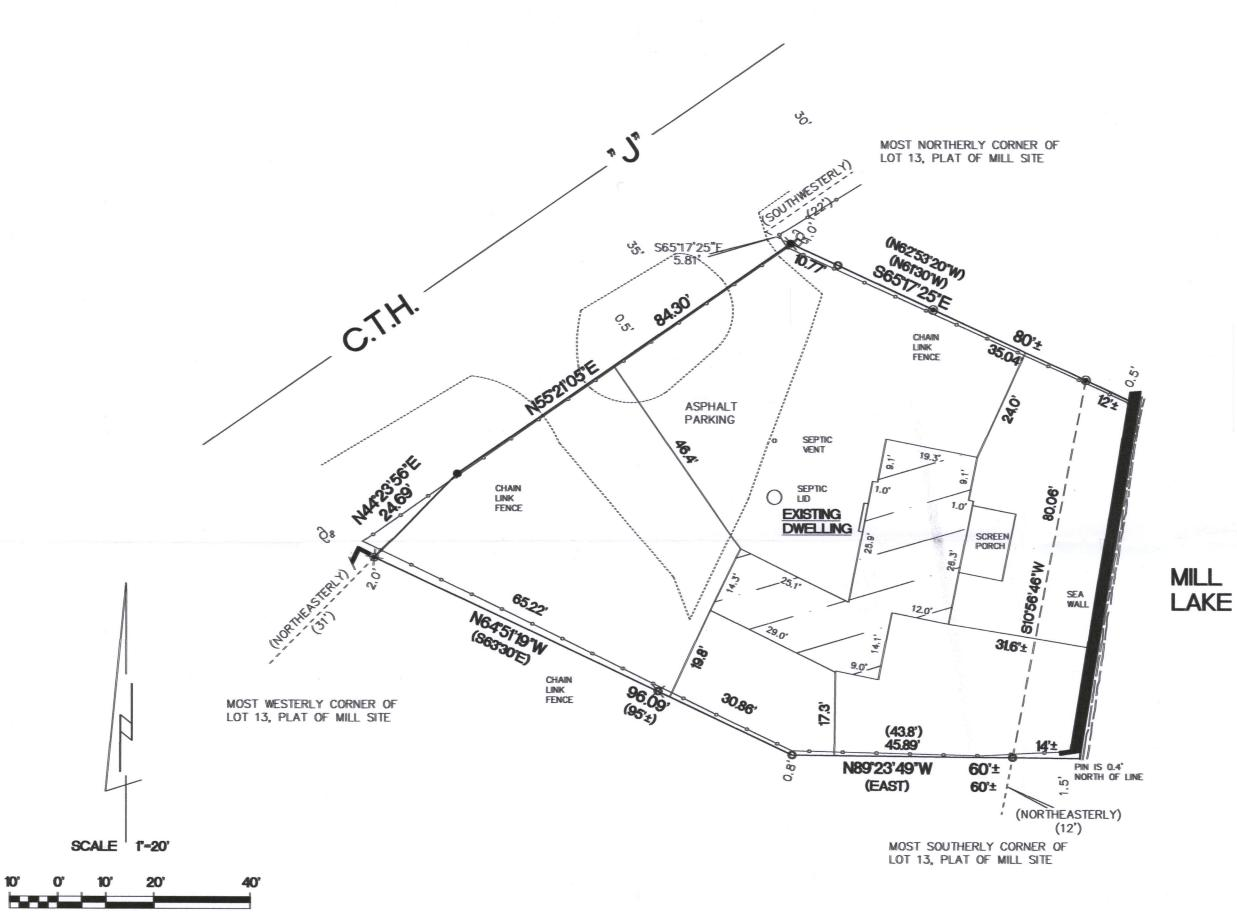
BEARINGS ARE REFERENCED TO THE WEST LINE OF THE NORTHWEST 1/4 OF SECTION 4-4-18, AND IS ASSSUMED TO BEAR NOO~10"30"W, (NAD27).
